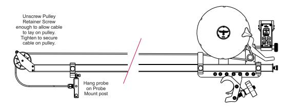
Press the Brake Lever and pull enough cable off of the Rotary Drum to allow the sensor to reach past the Pulley.
